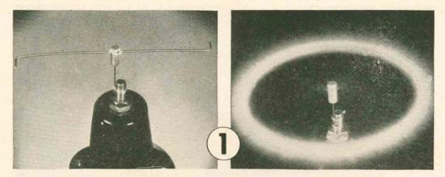
The spinner used in this experiment can be made of any light wire. Drill a small hole so that the metal will pivot on a pin attached to the high-voltage terminal. Shellac all but the tips of the horizontal wire.
