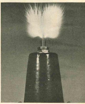
surface area—lots of it. If you try to conduct high-frequency currents through fine wires without enough surface area, the current will leap clear into the surrounding air, causing the inadequate wire to glow with a ghostly light. If you spell out a word with a continuous piece of 30- or 32-gauge bare copper wire, connect one end to the high-voltage terminal, and sandwich it between glass, the word will light up.
